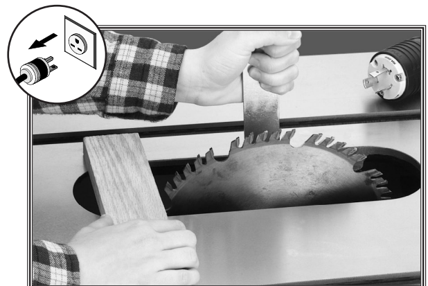
Figure 39. Using a scrap piece of wood to aid in tightening/loosening blade. Guard removed for clarity.
